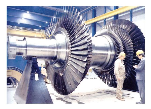
The principle design features of the straight condensing steam turbines are all structurally impulse, non-reheating, single cylinder type for power plants. The turbines use the advance 3-D technology for through flow path. The units are quite compact in structural size, but with high performance.
