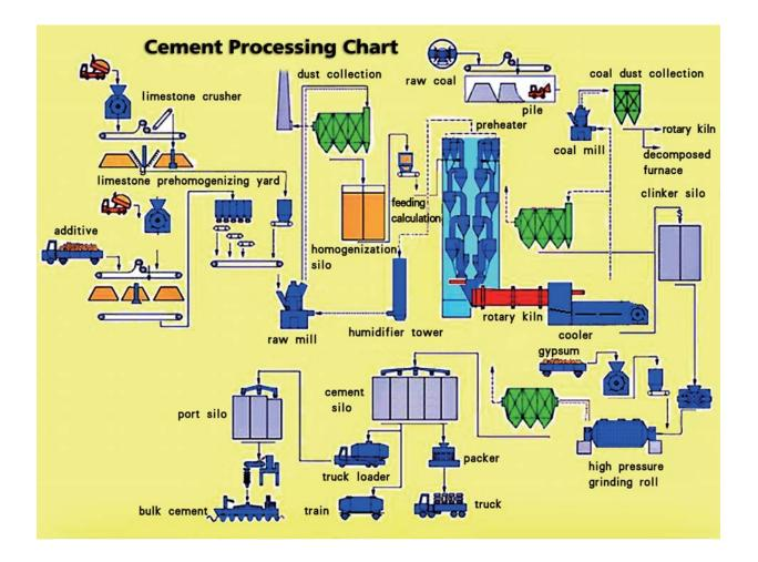
This information sheet describes the packaged equipment for a cement mill plant with the daily output capacity of 3,000 to 10,000 tons, or roughly one to three million tons per annum. Essentially, the package consists of the main components of cement mill equipment; plus some auxiliary devices associated wit these main operating components.
